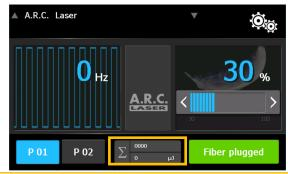
Pulse and energy counter for the documentation Counter is reset to zero by changing the probe
