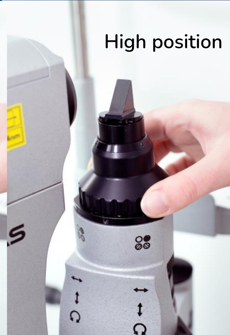
Illumination tower need to be in swing out position to laser
